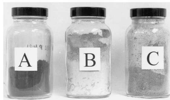
Fig. 1. Powder mixes, A (iron oxide and MCC) with clear glass wall, B (iron oxide and magnesium stearate) and C (iron oxide and titanium dioxide) coating the glass walls of the containers.
