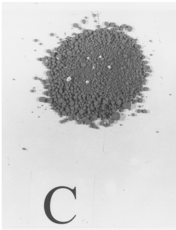
Fig. 2. Spheroids formed in mix C containing iron oxide and titanium dioxide.
